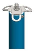
A Triple Swivel Tie-Off on the Upper Mast Section provides a means for securing an SRL/lanyard which is connected to the worker's safety harness. Anchorage relies on the engagement of the Swivel Tie-Off with the Boom Pin & Upper Mast Section. This engagement is designed to arrest motion
