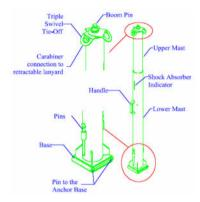
The Upper Mast Section rests on a Shock Absorber installed on the inner side of the Lower Mast Section. The Upper Mast Section is pinned to slide along the slots provided on the Lower Mast Section. The Lower Mast Section is pinned on to the SafeHold Anchor Base.
